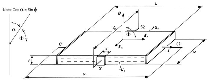
Figure 2. Schematic of a Hall chip<sup>(7)</sup>
